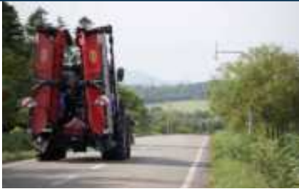
For transport, BX belts are positioned well within the cutting units.
