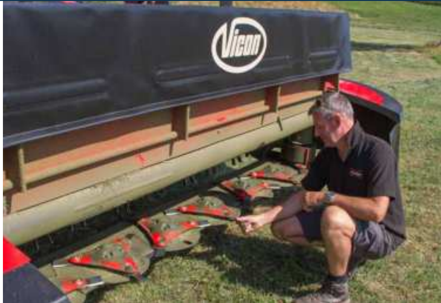
Front cover is opened into a vertical position for easy access.
