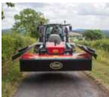
Hydraulic folding of FlexProtect guards (optional).
