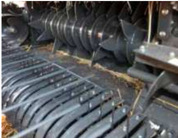
PowerFeed intake system.
