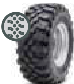
Bibload tread The Bibload tread offers high level of running smoothness and high mileage due to large ground contact area. Furthermore, the staggered tread blocks ensure optimum traction. The tread is further characterised by high wear resistance.
