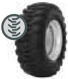
EM treads Thanks to the almost parallel lamellas, the EM tread is particularly well suited for loose ground such as sand, soil or gravel. Thanks to the high thrust transmission, this tire has a large footprint and runs very smoothly on the road.
