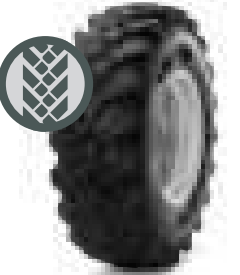
MPT tread The MPT profile offers the perfect combination of good traction on uneven ground conditions as well as fast road crossings.
