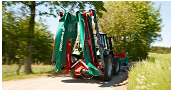
Vertical transport position for good weight distribution.
