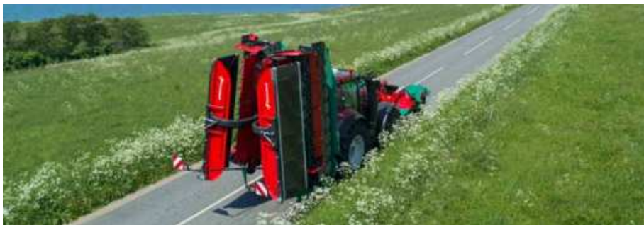
For transport, BX belts are positioned well within the cutting units.
