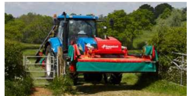
Foldable sideguards ensure narrow transport width.
