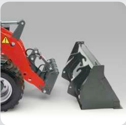
Efficiently change attachments. Thanks to the hydraulic quick-change system, attachments can be readily exchanged. Your Weidemann machine is therefore always ready for use. This increases productivity and profitability.
