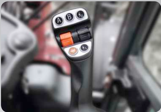
The joystick for the 1880. The joystick becomes an all-rounder, thereby increasing the machine's ease of use. In addition to the functioning of the 3rd proportional control circuit that can be activated via the joystick, the continuous operation of the 3rd control circuit can be activated via the rocker switch – by moving the thumb wheel (also in both directions). The optional function of the 4th control circuit can also be operated proportionally via the joystick. Both electrical functions can also be operated on the joystick in a detenting or latching manner. Both electric functions are independent so that they can be individually configured by the operator.
