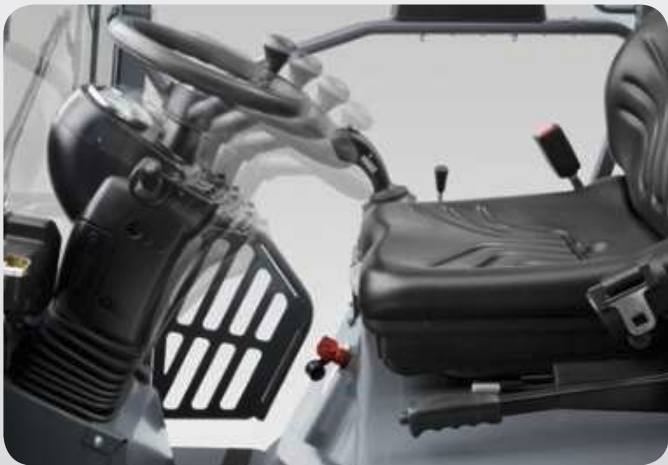
Adjustable steering column. Thanks to the adjustable steering column, you can adjust the operator's cab to your physical dimensions. By adjusting the various operator's controls, you can achieve a completely ergonomic working area.
