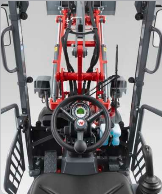
Good all-round visibility. The operator's canopy/cabin provides an excellent overview of the attachments, the immediate working area, and the entire machine surroundings.
