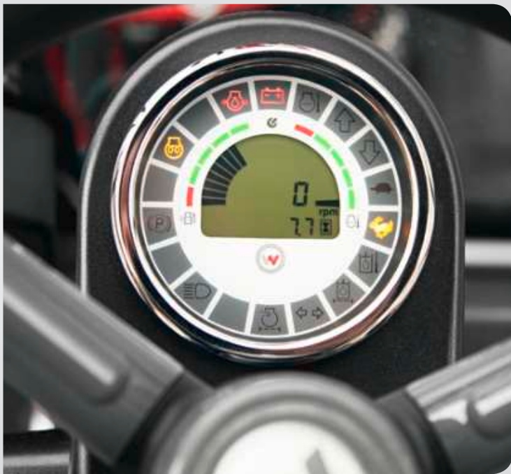
The main functions always in sight. Thanks to the digital display, you have a good overview of your machine. In addition to temperature, tank filling, or operating hours, active functions (e.g. electrical functions, the continuous operation of the 3rd control circuit or the activated differential lock) are displayed in the cockpit (varies depending on the machine type).
