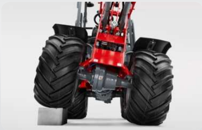
The backbone of the Weidemann design: the legendary articulated pendulum joint. Weidemann Hoftracs® always run with all four wheels on the ground – in any situation and in any ground conditions. Because the front and rear carriage can oscillate self-contained of each other, they react sensitively to every unevenness. The benefits: you always drive with maximum traction; no power is wasted.
