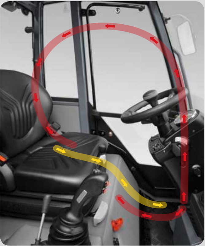
Comfortable working environment. An excellent working environment thanks to an efficiently working heating and ventilation system featuring a blower, fresh air filter, and well-placed air nozzles. In warm temperatures, an air-conditioning system is recommended (available for 1880).
