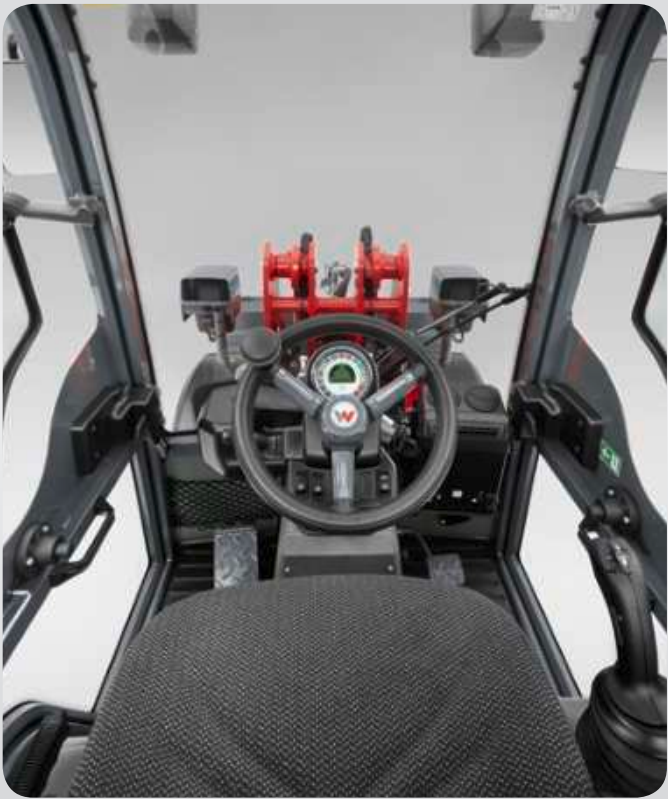
Ventilation as required. The cabins feature large, wide-opening doors on both sides. Depending on the cabin type, the upper window can be folded up completely and locked. A gap ventilation is also possible.
